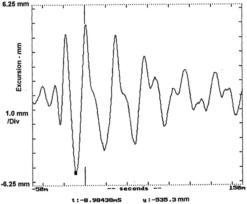
**Figure 2.** Time record over 200 ms of the excursion of a 160 X 231 mm (6 X 9 inch) automotive woofer in an infinite baffle driven by a music sound source just below clip point of the intended (15 watt) amplifier. Excursion to  $\pm 5$  mm was repeatedly observed with moderate audible distortion.
