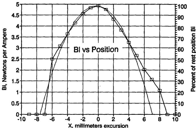
Figure 8. BI versus position for the 6 X 9 inch automotive woofer also showing the quadratic approximation.
