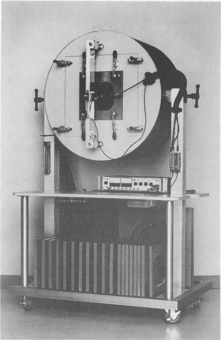
**Figure 5.** Overall view of the drive-unit measurements at excursion workstation. The cylindrical chamber rotates through  $180^{\circ}$ .
