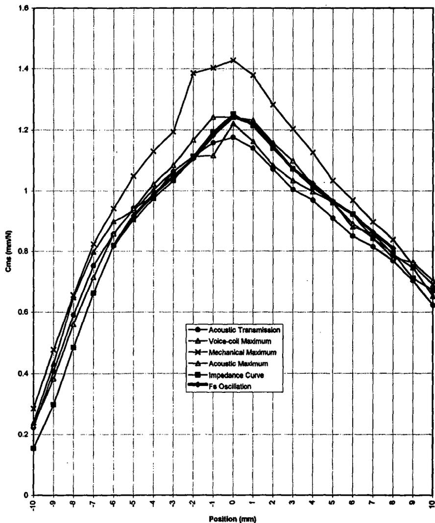
Figure 7.  $C_{MS}$  of a 178 mm woofer measured by six different techniques. The preferred technique,  $F_s$  oscillation, shown by the heavy line could only be applied between -6 mm and +8 mm for this long-travel suspension. The other techniques extend the measurement range and confirm each other reasonably.
