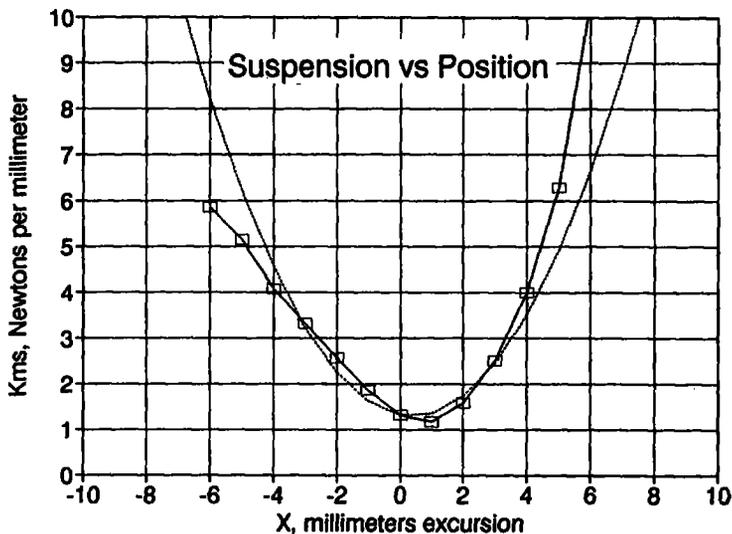
Figure 9.  $K_{MS}$  versus excursion for the 6 X 9 inch automotive woofer showing the quadratic approximation. The coefficients of the terms of the quadratic for  $K_{MS}$  and BI are used to predict distortion.
