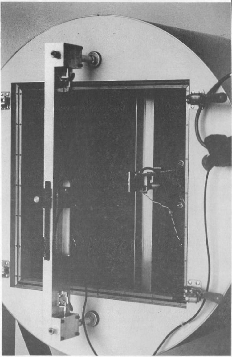
**Figure 6.** View of the laser position transducers and the interior of the test chamber.
